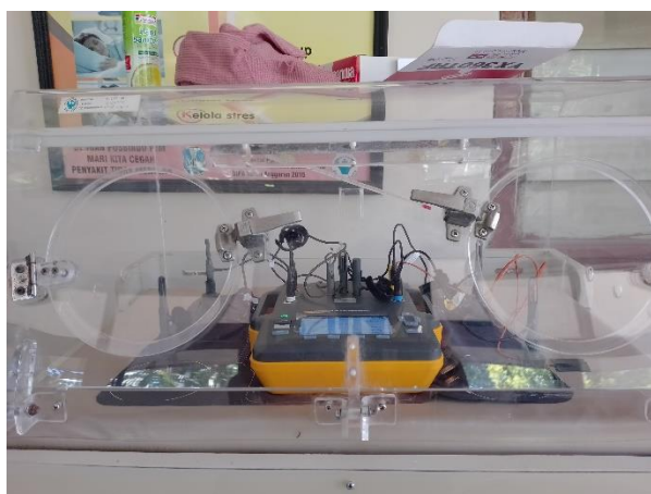
FIGURE 8. Measurement process using an incu analyzer
