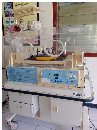
Figure 11. Measurement process using an incu analyzer
