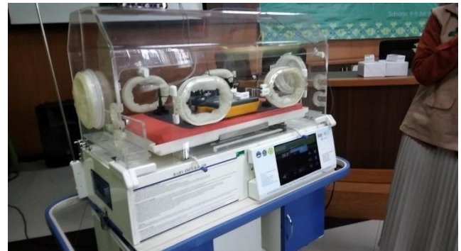
FIGURE 6. Simulating a baby incubator that has been equipped with telemedicine technology
