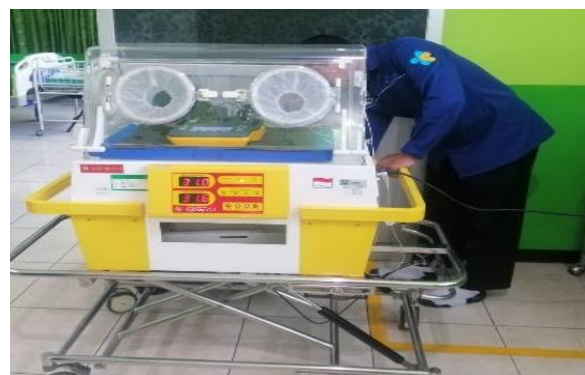
Figure 2 cleaning on infant incubator casing
